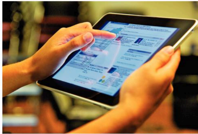
↑ A touch screen works as an input and an output device
