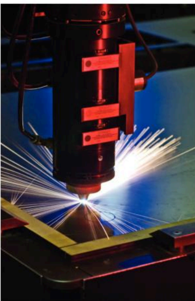
↑ A 2D cutter in action
