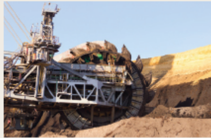
Figure 1.0 A giant bucket wheel excavator in use in an open-pit mine.
