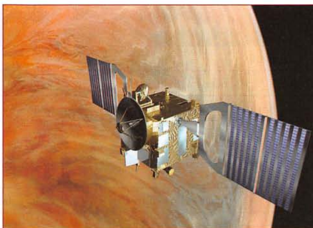
Figure 5.6 Image of the European Space Agency probe orbiting above the clouds of the Venus atmosphere. The Venus Express spacecraft was launched to study the thick atmosphere responsible for the intense greenhouse effect on the planet.
