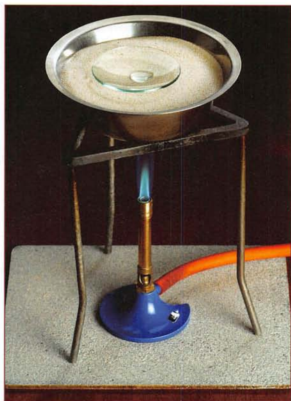
Figure 5.22 Evaporating off the water to obtain salt crystals. Here a sand tray is being used to heat the solution carefully.
