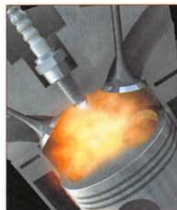
Figure 7.1 Computer graphic of the explosion within the cylinder of a petrol engine as the piston compresses the gases.
