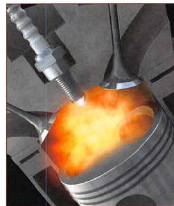
Figure 11.8 Computer image of an internal combustion engine cylinder. The piston (lower right) is moved up and down by the combustion (burning) of fuel. This image shows the fuel/air mixture being ignited by the spark plug.
