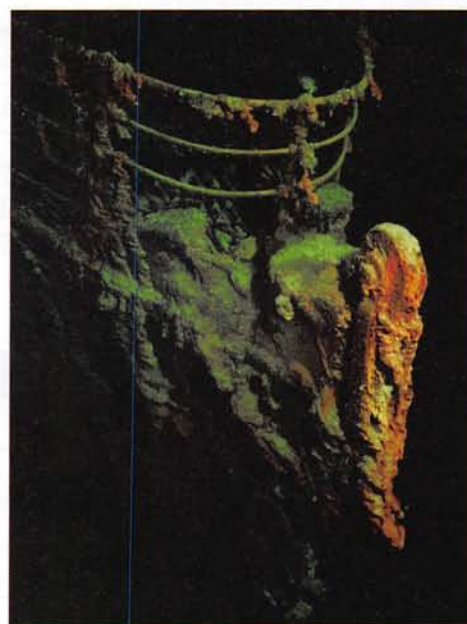
Figure 9.7 Photograph of the highly rusted bow of the Titanic taken from a submersible.
