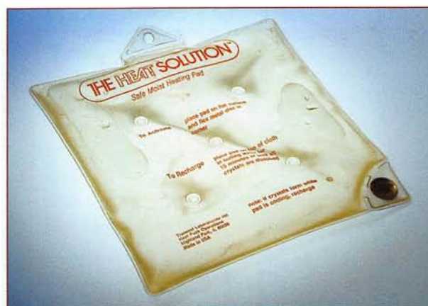
Figure 7.6 This hand-warmer depends on the heat given out when the solid crystallises out from the super-saturated solution in the warmer.
