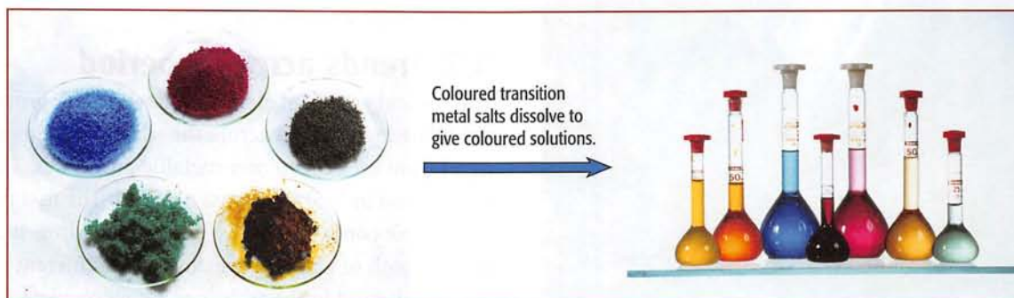
Figure 3.14 Many of the compounds of transition metals are coloured and, when they dissolve, they give coloured solutions.
