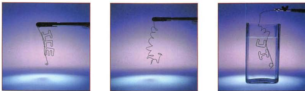
Figure 8.1 Restoring the shape of memory wire by heating: a the original shape of the wire, b the deformed wire, c the wire returning to its original shape in hot water.
