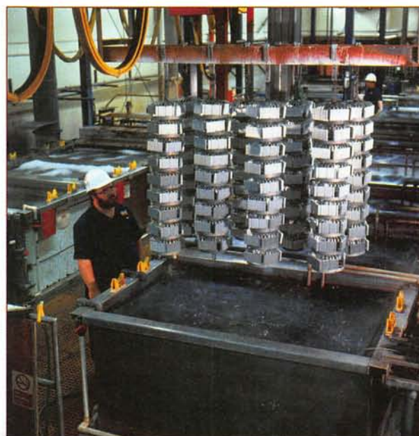
Figure 4.27 The industrial electroplating of metal objects.
