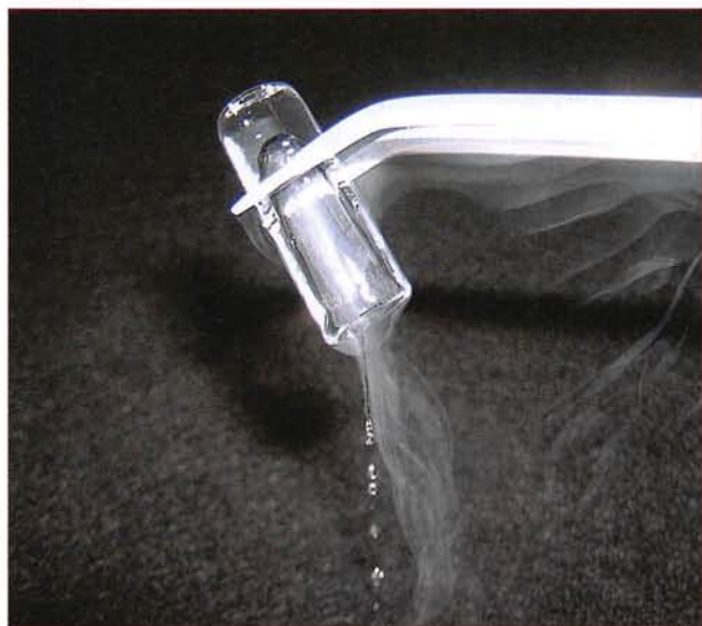
Figure 3.11 A small piece of rapidly melting 'argon ice' the melting point is -189^{\circ}\text{C} .
