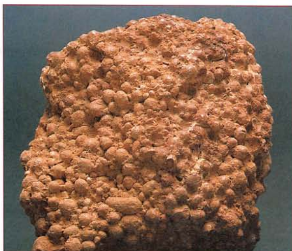
Figure 9.12 The major ore of aluminium is bauxite. It is usually mixed with iron(III) oxide, which gives the ore its brown colour.
