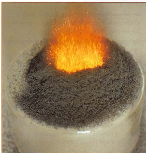
Figure 4.5 The decomposition of ammonium dichromate – the 'volcano experiment' – produces heat, light and an apparently large amount of powder.
