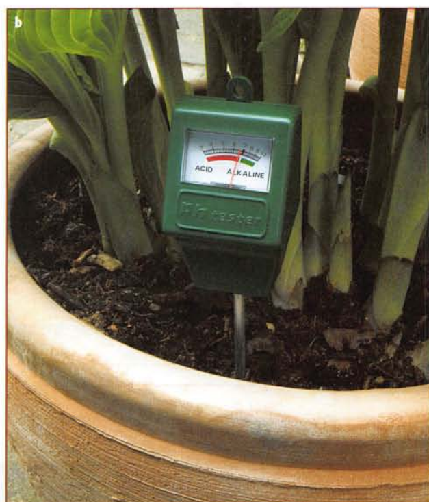
Figure 5.4 pH meters in use a in the laboratory and b for testing soil.
