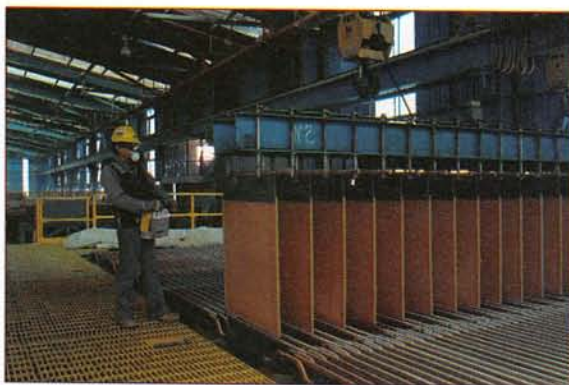
Figure 4.29 A copper refinery worker removes electrodes with extracted copper from an electrolytic bath in a Chilean copper refinery.
