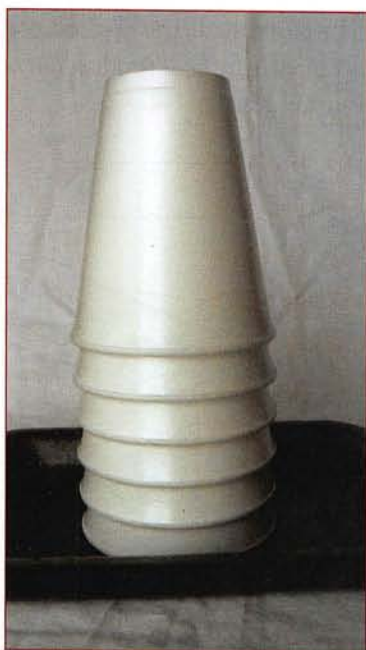
Figure 7.9 Polystyrene cups can be used as 'calorimeters' because of their good heat insulation properties.
