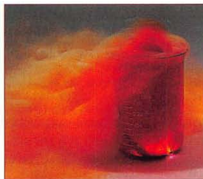
Figure 4.11 The reaction between aluminium and bromine is very vigorous, producing aluminium bromide. This experiment should not be attempted in the laboratory.
