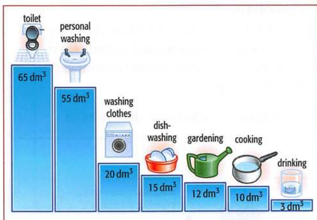
Figure 1.16 The main uses of water in a UK home. The numbers show how much water is used on average per person for each activity every day.
