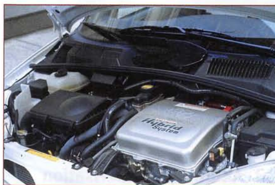
Figure 11.11 The Toyota Prius is a hybrid gas/electric car with low emissions. The battery charges while running on petrol and an on-board computer switches when petrol is low.
